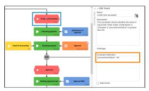
Designers can assign a **Field Name in Container** to form fields, that varies from the field's actual name (see page The Container Principle for further details). However make sure to use the **Field Name in Container** when defining the condition, since during the event verification the value in the data container will be used.
