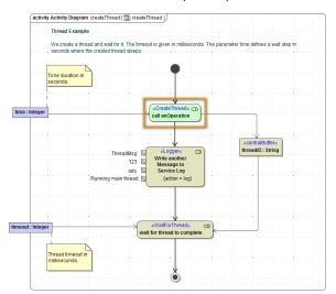
You can create a new thread using a Call Operation Action with stereotype << CreateThread>>.
