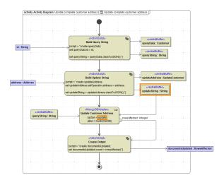
In this example, the address part of a customer document is updated. Depending on the structure of the update string, the complete address is replaced, or single address properties are updated. Refer to Building an Update String for more information on how to build an update string, and an example of the implications.
