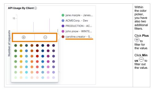
The value filter is applied to all diagrams in the dashboard:
