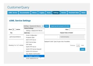
The default parameters are defined in the component diagram of the xUML service (see CustomerQuery example below). The connection is defined by a dependency between the composite named **CustomerQuery** and the SQL alias **customers**. The database user and password are defined in the tagged value **us er** on the SQL alias.
