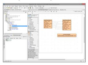
Activities implement the behavior of operations. Each class operation has to be assigned to its implementing activity diagram. When the operation is called, the assigned activity diagram will be executed.
