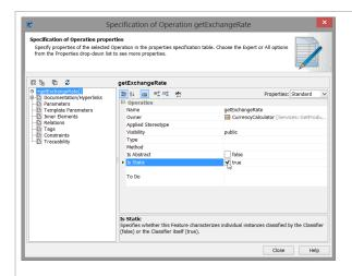
Double-click the Operation in order to open the Spec ification dialog. Set the Visibility to public. Then select the checkbox I s Static to set this option to t rue.
