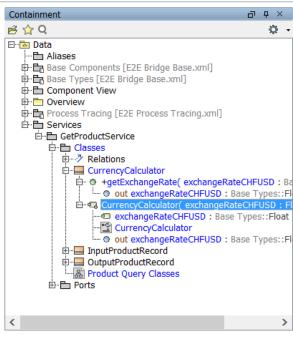
Expand the activity Curren cyCalculator in the containment tree. The activity has been created automatically and contains the activity diagram having the same name. MagicDraw uses the activity diagram name as default name for the activity. Furthermore, all parameters and activity parameter nodes are created automatically, according to the class operation parameters.
