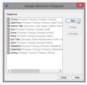
The Assign Behavior Diagram dialog displays a list of existing activity diagrams that can be assigned to the operation. However, this operation gets assigned a new activity diagram. Click the New button.
