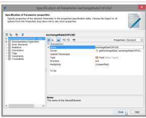
Assign the name exchan geRateCHFU SD, the type F loat [Base Types], and set the direction to out as the operation will return this parameter.
