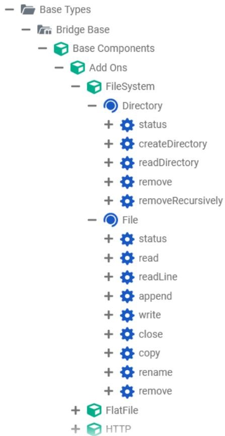
Expand the path to the Filesystem adapter in the service panel (**Base Types /Bridge Base /Base Components /Add Ons /FileSystem**).
