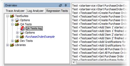
After running the test suite containing the logfile, the logged data is displayed in the content pane. The logfile is a normal text file and can be treated with any editor, e.g. for searching purposes.
