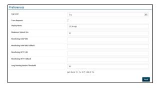
The service needs to be registered under **Monitoring SOAP URL**. If you have several BRIDGE instances, they can be configured as monitoring fallback, if there are problems with the main Bridge. Therefore, the Monitoring Service has to be deployed on the other instance(s), too.
